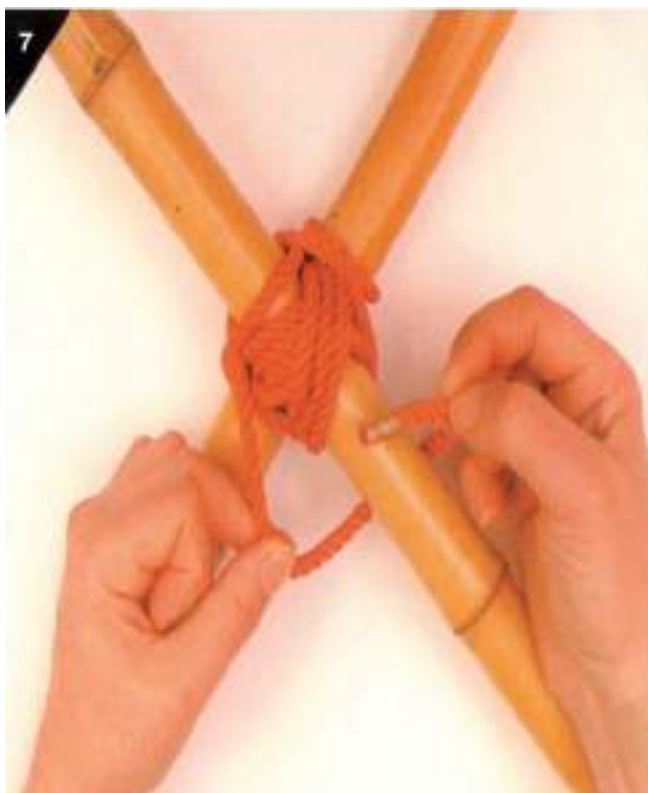
STEP SEVEN. MAKE TWO COMPLETE FRAPPING TURNS.
